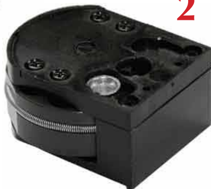
Image 2: Pellet inserted but not properly seated.
