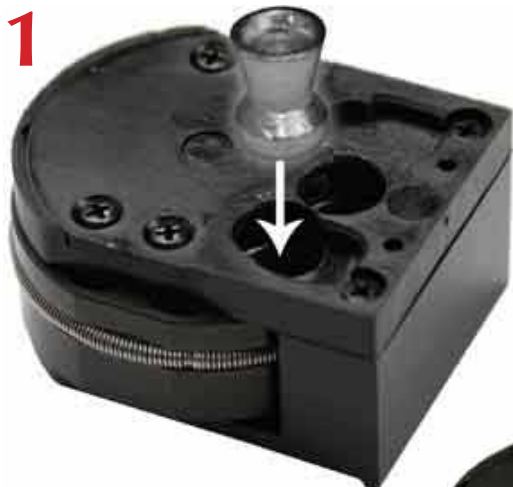
Image 1: Insert a pellet into the hole on the lower left.
